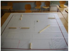
The lines mark positions for wooden barriers. Each set of lines (lines of the same colour) create a different setup on the field. Teams start their robot from the start and have to reach as many corners (black hexagons) without touching the wood in a period of 15 minutes.
